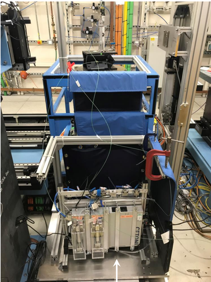
Pumps for injecting H 2 and brine and for the confining pressure and backpressure
